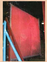
Exposed face of Fireshield test specimen, red hot after 4hrs of flame testing
